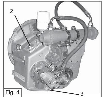
Remove the filler cap [2] and extract the oil level dipstick [1], as shown in the figure.
