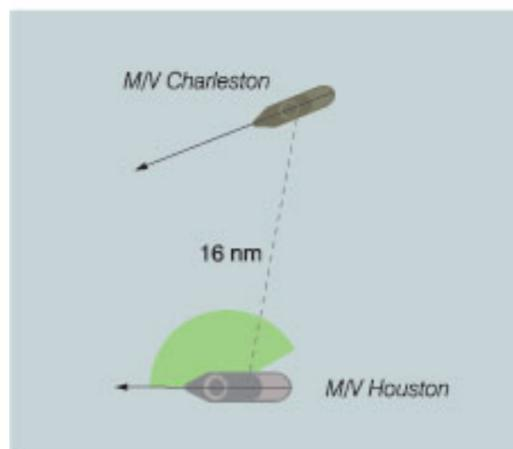
In this starboard quarter approach, the relative position of the vessels and configuration of navigation lights change over time. While the steering and sailing rules apply to vessels in sight, this scenario can still lead to confusion as to whether this is an overtaking or crossing situation under certain circumstances. Never assume the other vessel shares your view of which rules apply. Be prepared to take evasive action.
